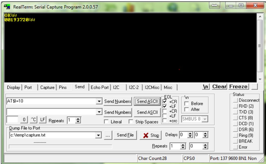
5.7 Clear first text box and type `AT$SF=544553544D455353414745` with +CR and +LF ticked. This is the command to send a message and the message (TESTMESSAGE) here is shown as Hex value in ascii.
